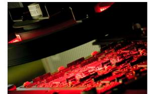
Consistent high quality is paramount in the drive to deliver zero defects on PCB assemblies. CT employs the latest in AOI systems to confirm that the parts and assembly are correct. The latest generation multiple camera machines are also capable of reliably inspecting solder joint quality!
